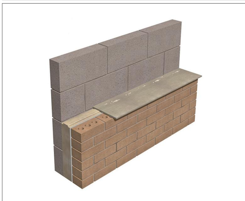
14.11 The boards can be cut, using a sharp knife or fine-toothed saw, to fit openings, eg around windows, doors and airbricks. It is essential that cut pieces completely fill the spaces for which they are intended and are adequately secured.
