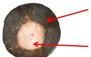
Kiln Dried Pine offers 100% Sapwood penetration of the Chemical treatment, not possible with Spruce. Sapwood is the part of the timber which is non durable and most susceptible to fungal and insect attack it needs to be protected.
